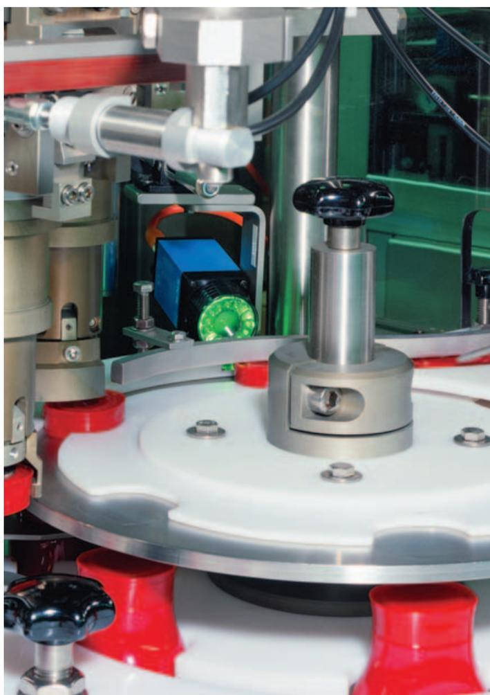
◀ Specialist for position and shape: the ICS checks the orientation of bottle tops in an automatic bottling plant.
