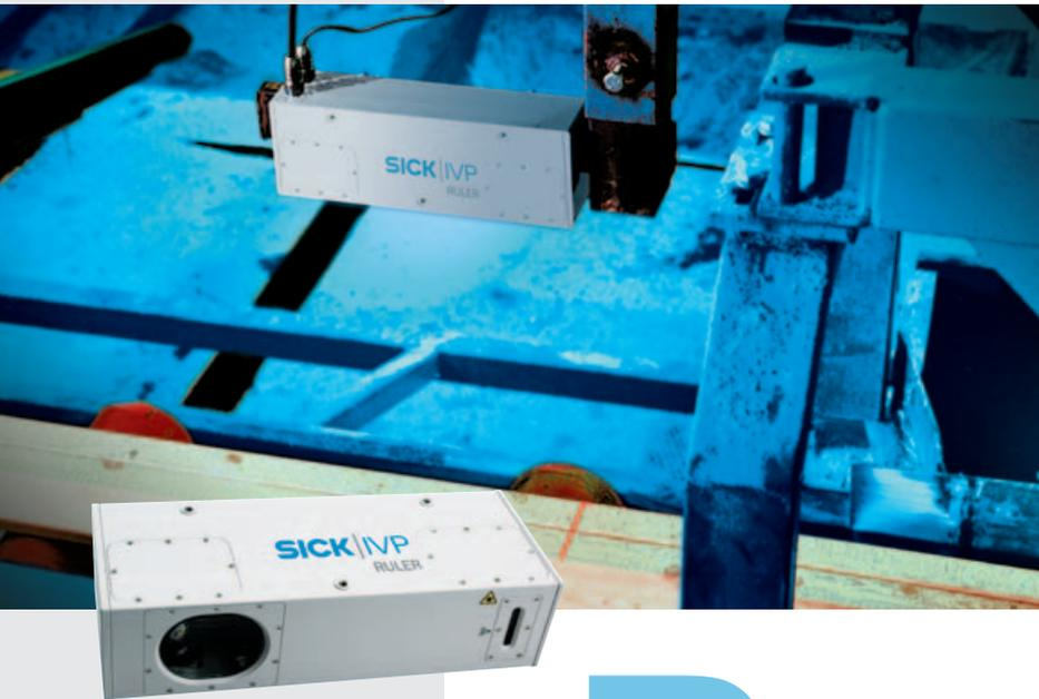
Ruler E is a camera with in-built laser and optics for a predefined field of view, which makes it very easy to install. The data output from the Ruler is calibrated world coordinates (x, y, z) in millimetres which are delivered on a high speed Gigabit Ethernet interface to a hosting PC. Application development is made in a high level VB .Net or C/C++ programming environment.
