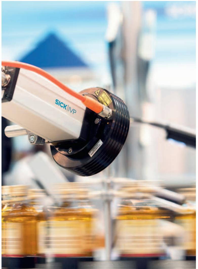
► The flexible IVC-2D camera can easily inspect many features simultaneously - in this case cap position, fill level and label.
