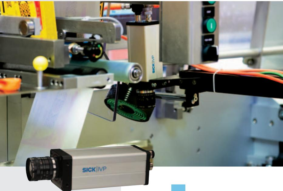
Top-Performance to meet production demands of tomorrow: A powerful processor, optimized pixel processing in FPGA and advanced machine vision tools ensure that you never fail to inspect the object in time, even at the highest production speed.
