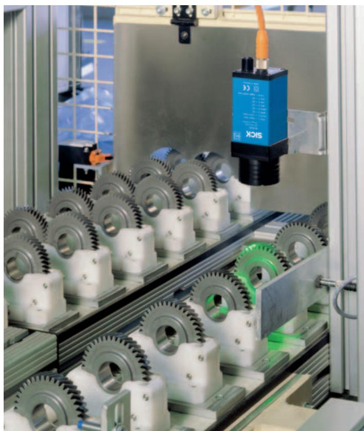
► Is a gear tooth missing or was the surface incorrectly treated? The ICS already meets the requirements of different testing processes.
