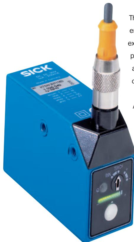
Thanks to the three-colour-LED-technology, the optimum emission colour is automatically selected depending on the existing contrast. Furthermore, the precise 2-point-Teach-in procedure is provided, where the gray values of the mark and the background are taught-in. The sensor sets the optimum switching threshold automatically.
