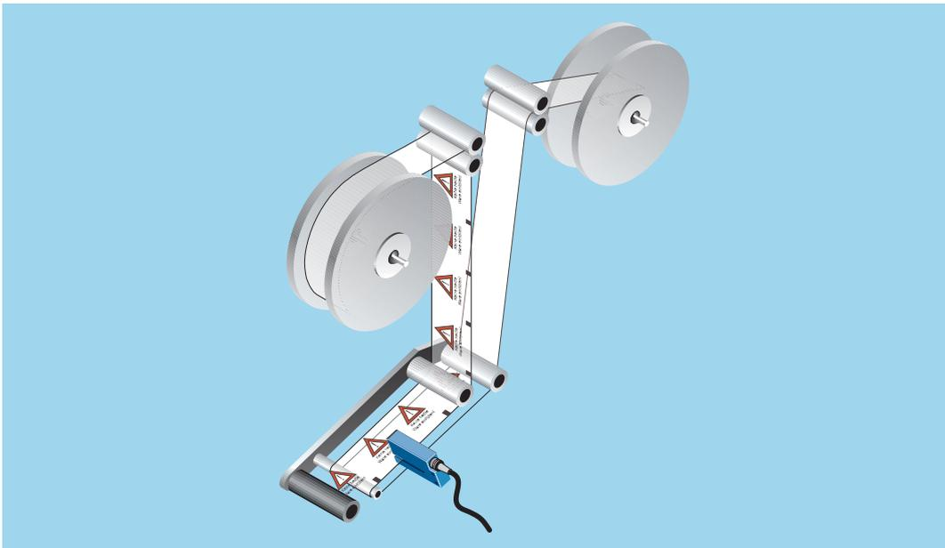
◄ Labels can only be cut and punched if printing and control marks can be accurately detected. Fork sensors are used to ensure that everything runs smoothly and reliably.
