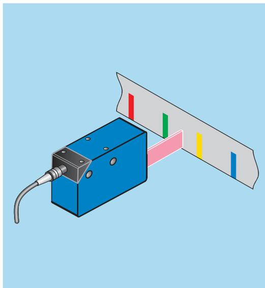
◀ Print mark control with the CS8: each channel corresponds to one coloured mark.
