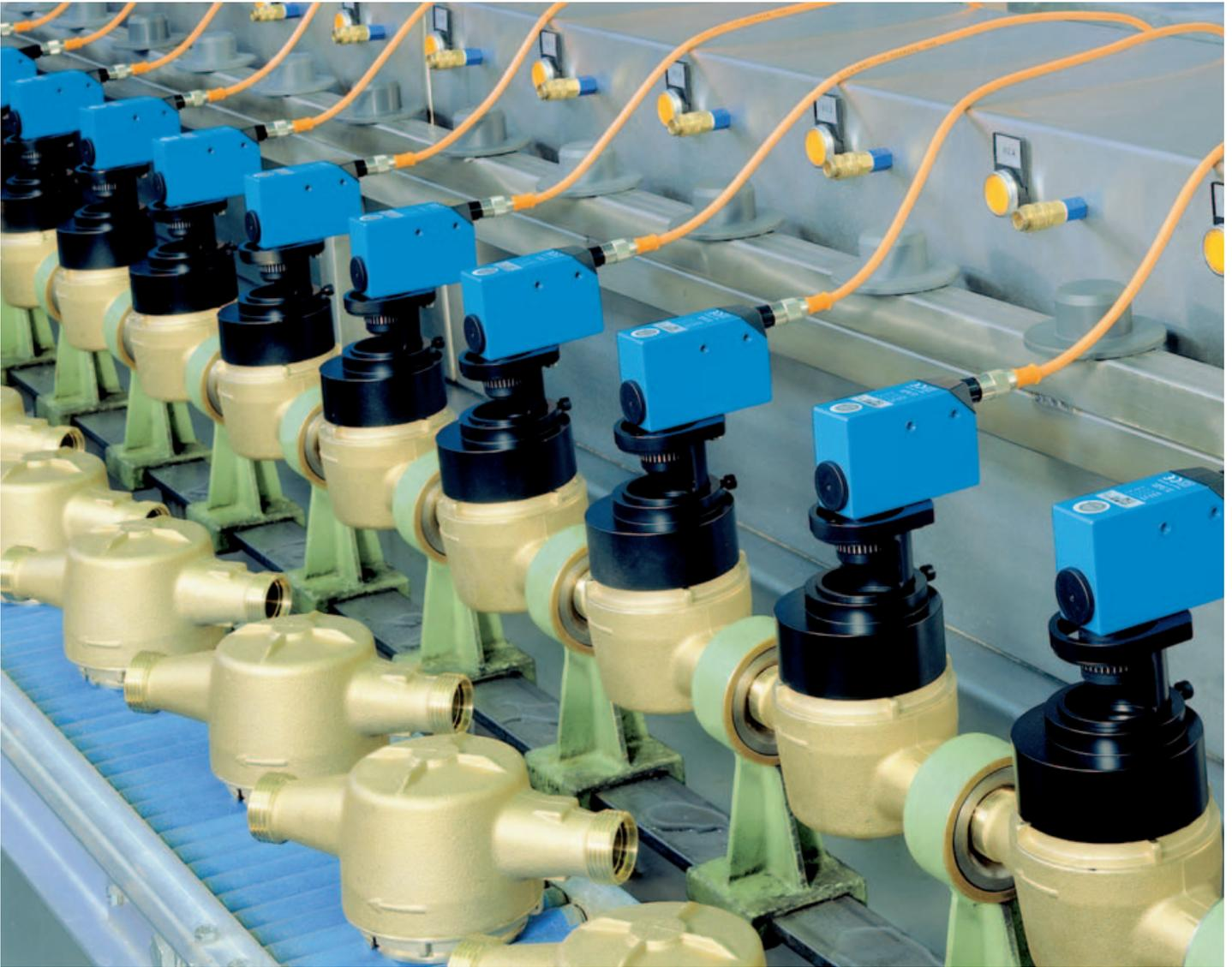
▲ KT contrast scanner in water meter manufacture
