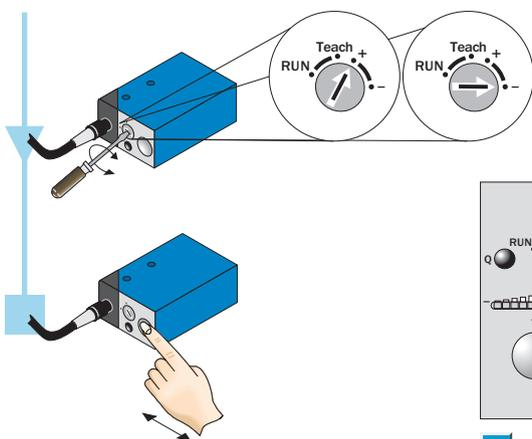
■ Adjustment of the switching threshold via position +/- and pressing of keys.
