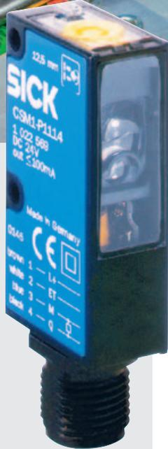
The choice of color tolerance is determined during the Teach procedure. The CSM offers the choice between “medium”, “fine” and “coarse” settings. Upon pressing the Teach-in button, the transmission light changes from “green” to “blue” and then to “red”. Depending upon which color of the Teach process is triggered, the corresponding color tolerance is automatically set. The simplicity of this procedure characterises the CSM.
