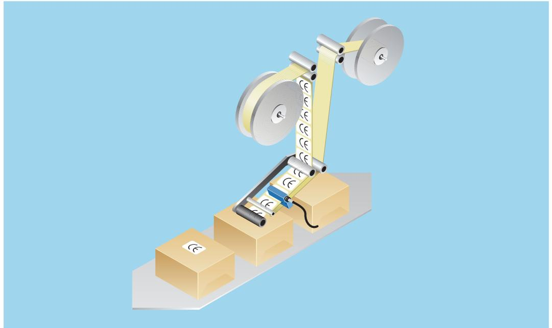
▼ The fork sensor reliably detects double sheets on conveyor belts carrying material to guillotine cutters.
