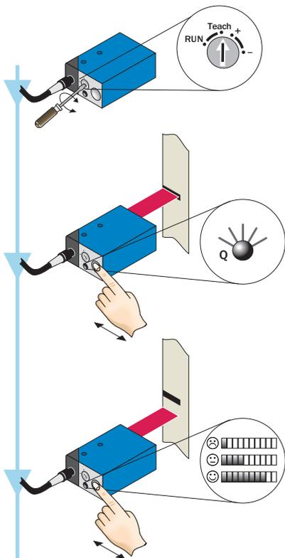
■ After the first Teach-in procedure, the red transmitter light and the status indicator blink and signal that a second Teach-in procedure must be triggered.
