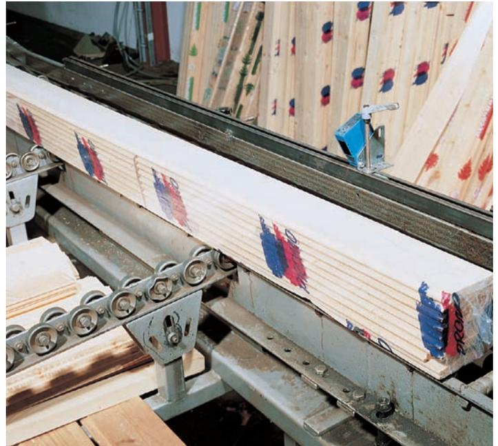
▲ A WT 260 photoelectric proximity switch controlling a commissioning system used in the wood-working industry.
