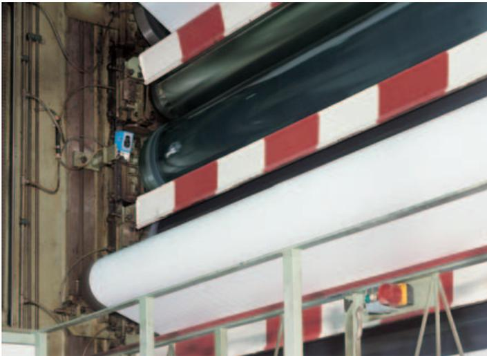
▲ Extreme operating conditions exist in steel making plants – the WT45 photoelectric proximity switch is ideal for many applications, such as detecting metal sheets before they are wound onto coils.
