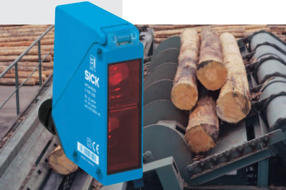
Due to their easy operation, the devices are quickly ready to operate. The screw connections and device plugs, which are rotatable through 90°, provide optimum cable entry in any mounting position. Moreover, the W 34 series is compatible with the W 36 series from a mounting viewpoint. All W34s are available either as a DC or DC/AC option.
