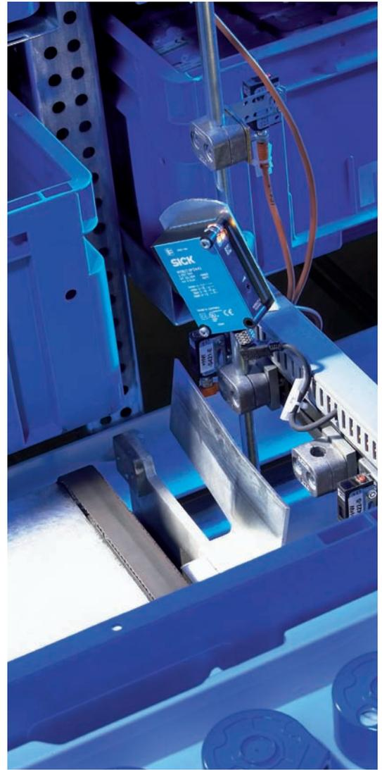
▼ The WL27-3 photoelectric reflex switch reliably detects the pallet wrapped with foil.
