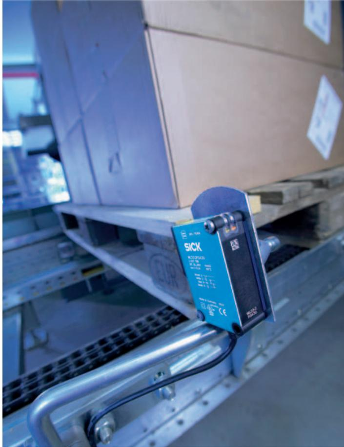
▼ WL23-2 photoelectric reflex switch detects very variable material to be conveyed, e.g. beverage boxes.
