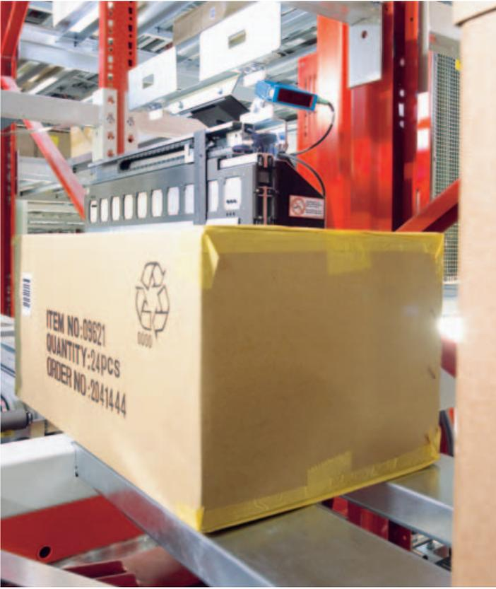
◀ The WT34 photoelectric proximity switch stands out for its large scanning distance with regard to checking whether second or backward storage bays are occupied.
