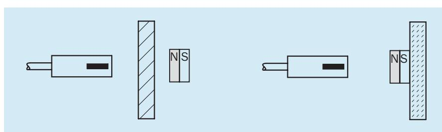
**Mounting on magnetizable material**
