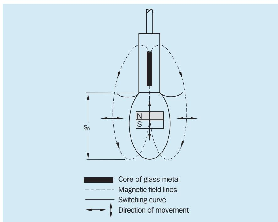
Case 2: The sensor responds if the magnet approaches the switching curve laterally. If the sensor leaves the switching curve, the sensor switches back again. This principle is largely used for magnetic cylinder sensors.
