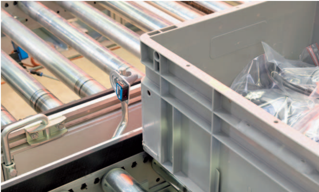
▶ WT100 photoelectric proximity switch with background blanking detects reliably conveyed objects.
