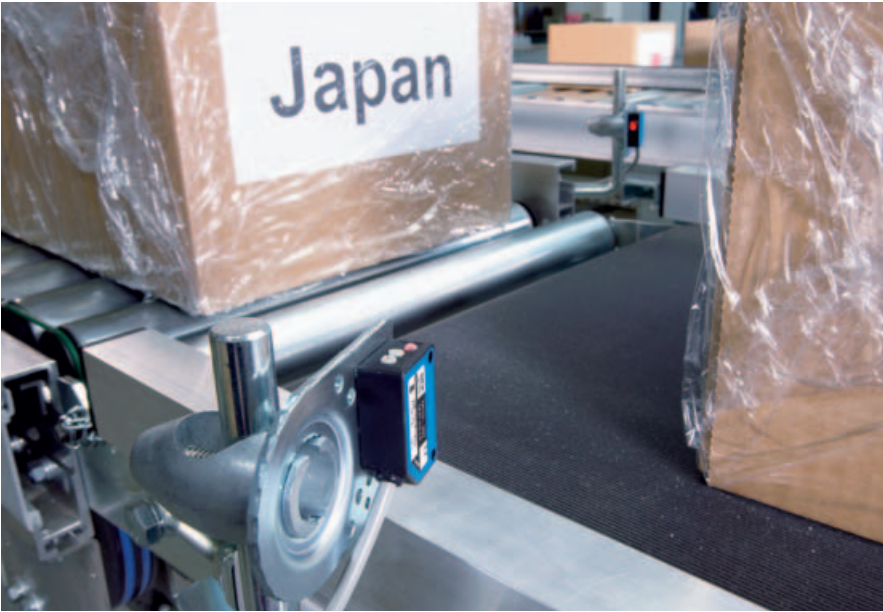
◀ WS/WE100 through-beam photoelectric switch detects filmed objects safely.
